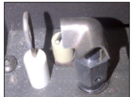
Figure 13: Proper Pilot Position
