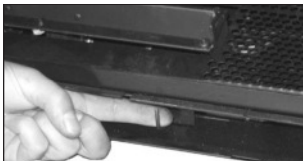
Figure 5: Adjusting the venturi air setting.
