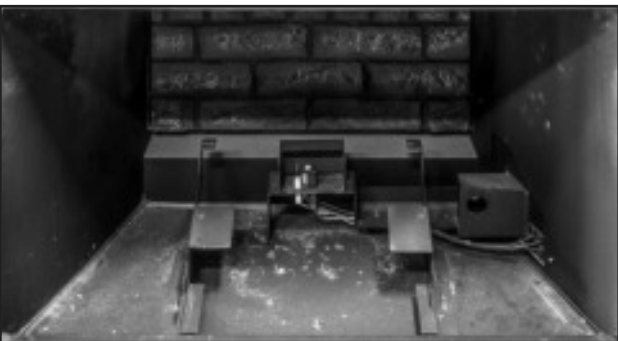
Figure 44: Lift the burner off the mounts and pull it out of the inlet box. The unscrew the panel brackets (T20's) from each side of the baffle to remove the left and right side liners.
