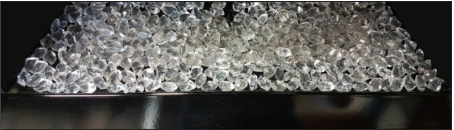
Figure 33. Glass Media Installation
