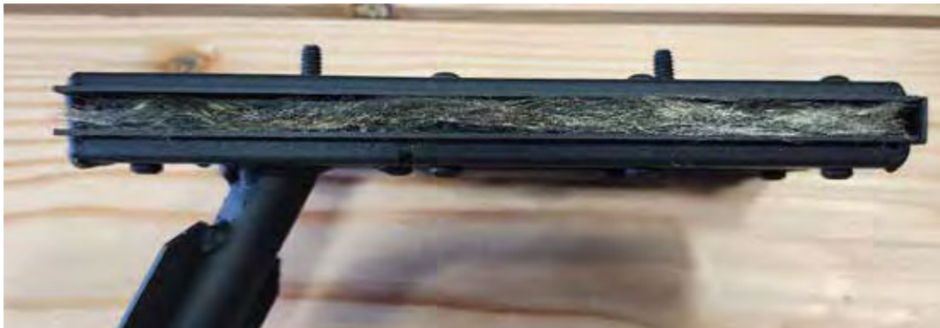
Figure 84: Nickel Strands Installed in Burner Slot
